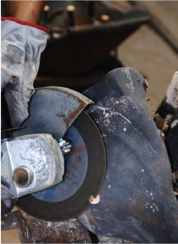
2. Removing gates & vents
